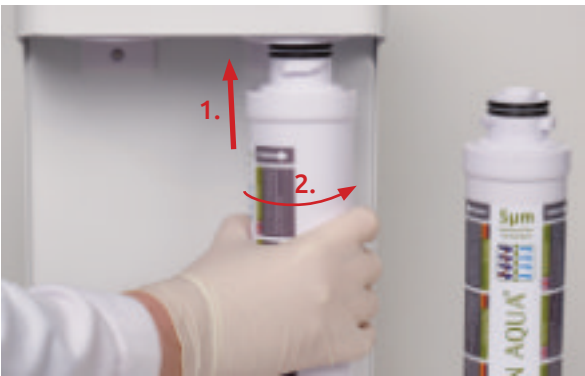
Press the new activated carbon post-filter unit into the filter head and turn them 90 ° clockwise.
